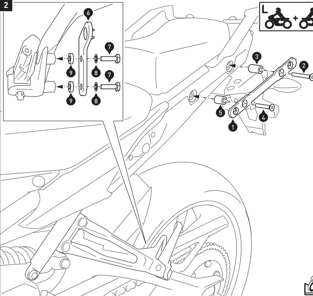
Attach on both sides of the vehicle the mounting brackets (1), as shown in the drawing.
